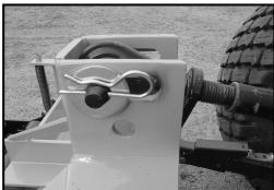
Industry Exclusive: 3-Point Center Link Control Choose the setting that's right for you. Rigid setting for transport and increase, lifting height. Float setting for machine operation and ground following action.
